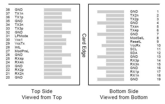
Figure 2. Electrical Pin-out Details
