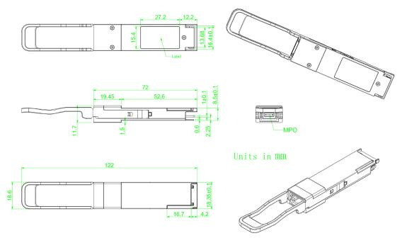
Figure 9. Mechanical Specifications
