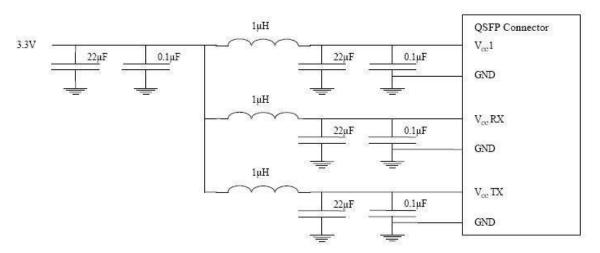
Figure 3. Host Board Power Supply Filtering
